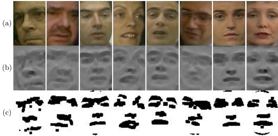
Figure 5: (a) Sample faces, (b) result of intensity normalization, (c) facial features after intensity thresholding.
