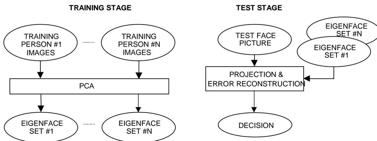
**Figure 1.** Block diagram of the self-eigen approach for face recognition
