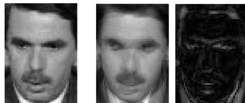
Figure 6. Decoded (reconstructed) image José Mari . Left: original image. Center: reconstructed image. Right: Error image.
