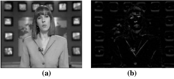
Figure 3. (a) Original grey scale image after erosion;(b) Vertical close of (a).
