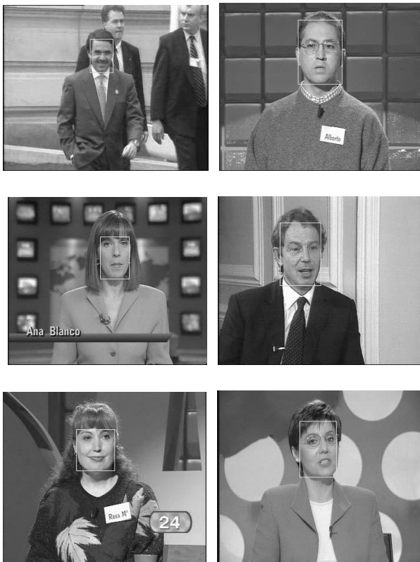
Figure 4. Faces automatically detected and recognized by the proposed system
