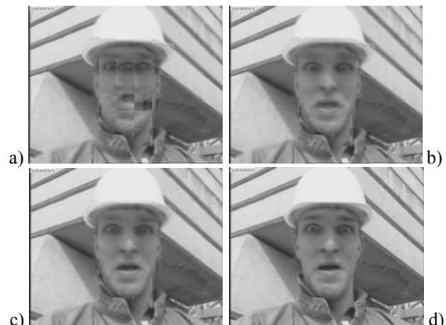
Figure 4 Frame 93: a) MCTI b) MCTI with the 3D model rendered on top c) decoded picture (MCTI + model + parity bits) d) original picture
