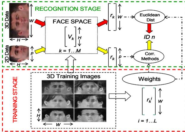
Fig.1 P<sup>2</sup>CA: General Block Diagram
