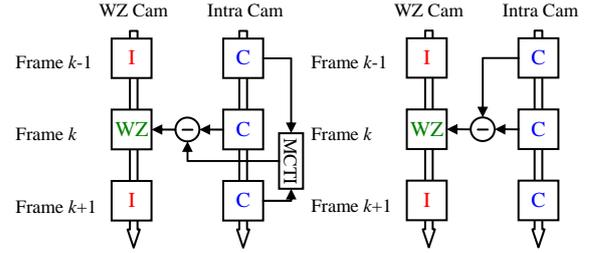
Fig. 3. Structure of the PMCE and PNFE techniques.
