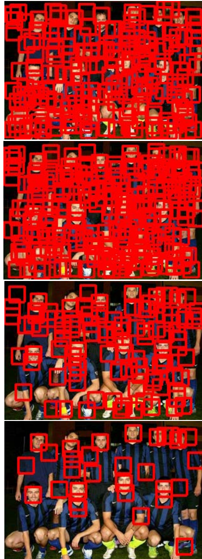
Figure 8: Adaboost Results. (From Top to Bottom are the outputs of the 1 st , 2 nd , 3 rd and 4 th stage Adaboost cascade scheme)
